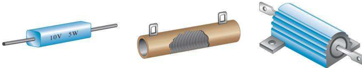
(a) Film resistor showing spiraling technique
