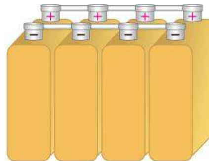
(b) Parallel-connected cells increase current capacity.
