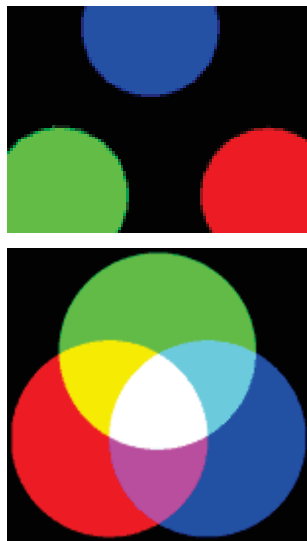
Figure 3. Additive colour mixtures of blue, green and red to produce cyan, magenta, yellow and white.
