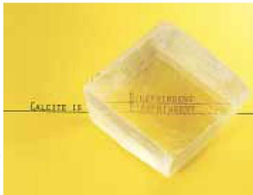
Figure 38.35 A calcite crystal produces a double image because it is a birefringent (double-refracting) material.
